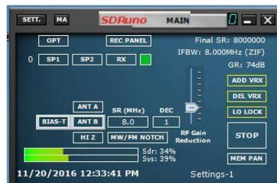
RSP1, you will see the window on the left. If you use an RSP2 you will see the window on the right. The Main difference between the two is the buttons for antenna switching. To start SDRuno, click **PLAY**.
