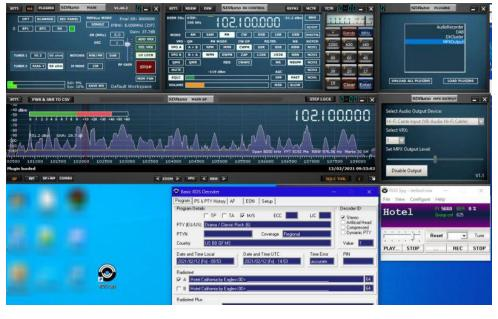
Turn on the SDR and find a tune to a station that uses RDS. Then double click on the RDS Spy icon on your desktop and load RDS Spy. Go to the "Configure" tab, select RDS Source. Make sure that Hi-Fi Cable Output (VB-Audio HI) shows in the Input audio device window and that Direct RDS/MPX (192khz) is ticked in the Sound Card Input Mode box. Then click okay.
